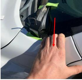
4. Once it is confirmed that the threads are engaged properly, reverse the bolt until the bracket has a small amount of play. Place the rubber pad in between the bracket and the fender. Trace the outline of the sides of the bracket and the top of the fender. Cut pad and remove adhesive backing. Adhere pad to inside of upper fender. Torque the bolt snug. Repeat steps 1 through 4 for the opposite side of the vehicle.
